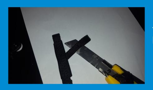
Use the Olfa or any flat knife and cut trough the sewing of the webbing on the brake pulley loop attachment.
