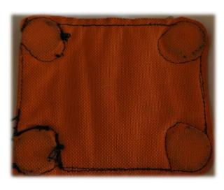
• Cut off the rear end (wrist) of the elastic working glove and sew it (without stretching it) onto one of the plates. This should be tight enough for most
